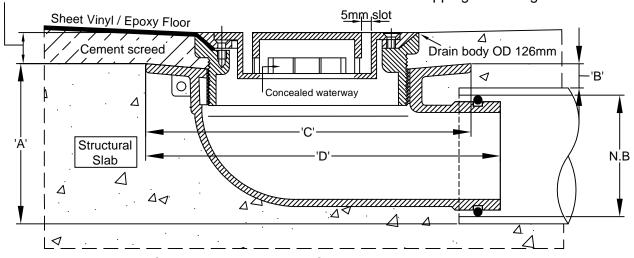
Spigot pushes into 65mm PVC or copper with o-ring connection, or connects to 50mm PVC/HDPE with no-hub coupling.
