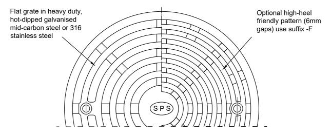
Load-tested to Class D of AS3996-2006
