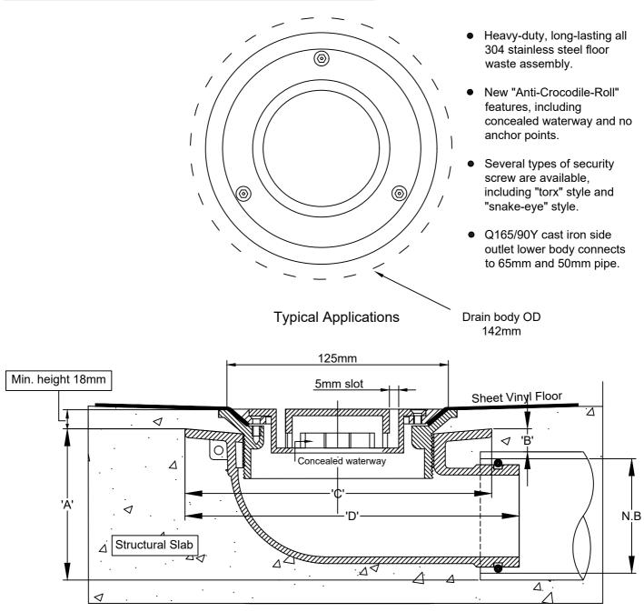
Spigot pushes into 65mm PVC or copper with o-ring connection, or connects to 50mm PVC/HDPE with no-hub coupling.
